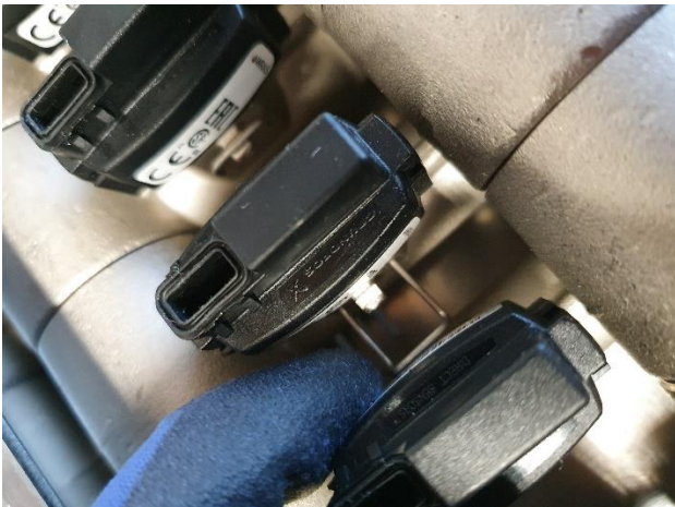
9. Push the locking pin back in. It may be challenging if it has been pulled out too far in steps 2 and 3
