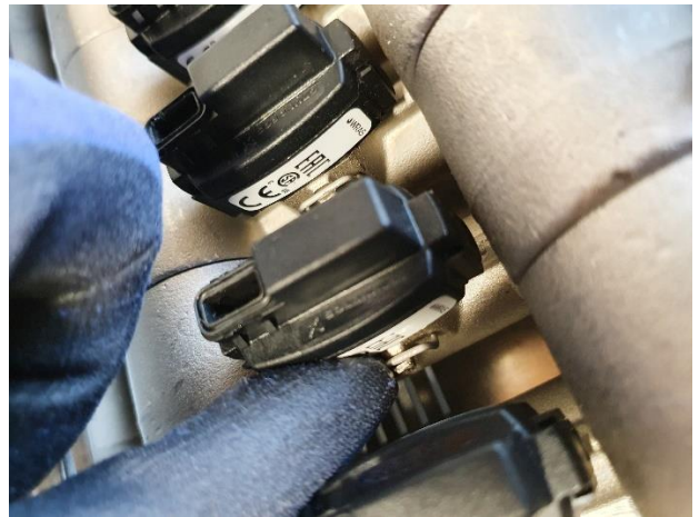
10. Push the locking pin all the way in. You will know that it is all the way in, when it is within the small gap of the hook on the piping.
