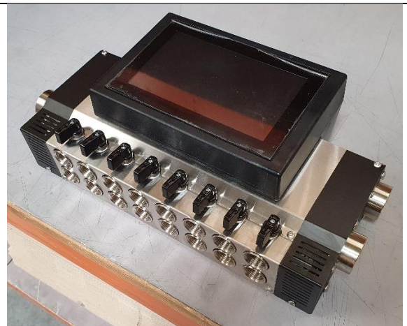
Incomplete 8 zone manifold
