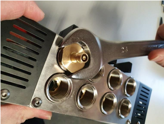
3. Tighten the fitting well, to ensure that the manifold does not leak.
