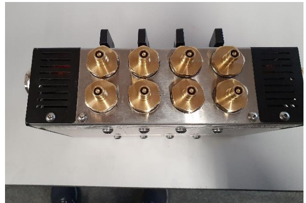
6. Finish mounting all of the fittings. Once that is done, the manifold is ready to be connected to your system.
