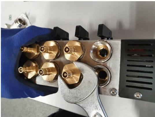
5. It is possible to fit the fittings in any order, but it is recommended to finish either the top or bottom row before starting on the other row.
