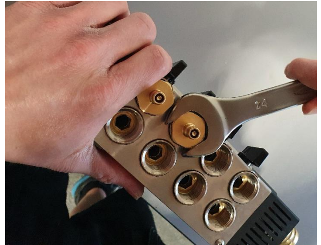
4. Continue mounting fittings for the rest of the channels
